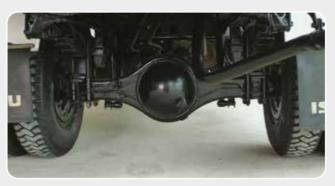
Bigger Rear Axle Capacity (Up to 6.6 ton) Greater axle load is durable for maximum loading and makes the vehicle ready for tougher conditions.
