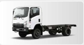
One Piece Straight Chassis Even load distribution ensures better stability for heavy usage and effortless body mounting.
