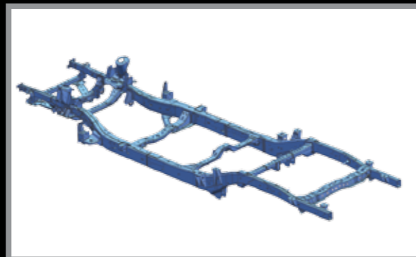
A stronger, durable yet lighter ladder chassis design for increased rigidity, safety and load carrying capacity.
