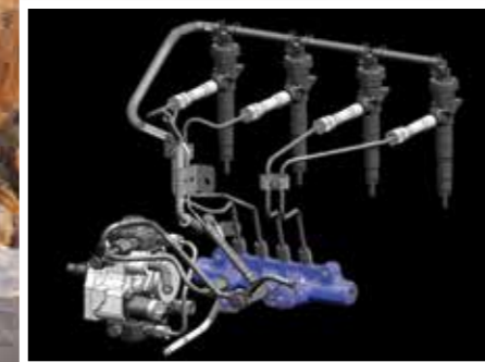
Improved high pressure common-rail fuel system.
